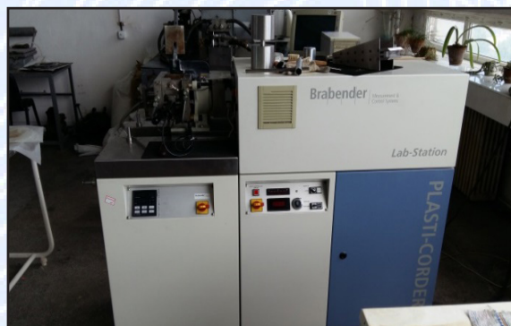
Fig. 69. Malaxor Plasti-Corder Brabender Mixer 350 E https://erris.gov.ro/Rubber-Research-Department
