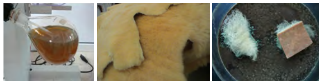
Nano-silver colloidal solutions (a) made for medical furs processing (b) and for the manufacture of a microbiologically resistant material (c)
