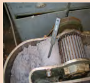
Leather waste paste in beating engine (discontinuous process)
