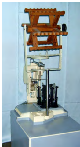
Prototype machine for manufacturing 3D parachute cord
