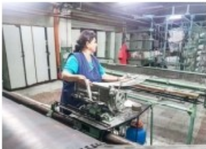
Fig. 1. Operatia de urzit in benzi
